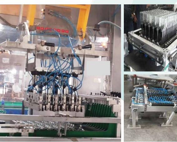
We design and consult on improvement packaging systems and also have been continuous (speed and simplified design/constru ction) such as pick & place, grippers, tray & wrapping and many such customized designs.
